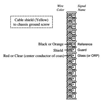
Some cables have connectors on the leads. Cut off the connectors, skin and tin the leads and then wire to the screw terminals on the boards
